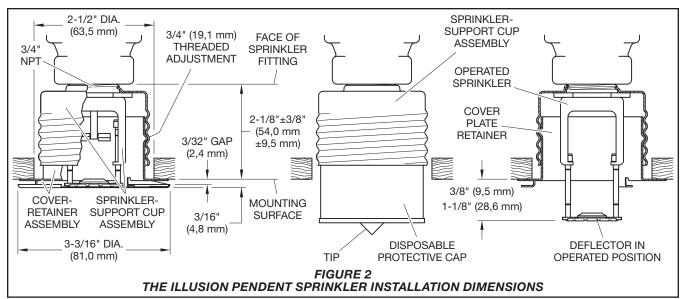
Do not attempt to compensate for insufficient adjustment in the sprinkler assembly by under-or over-tightening the sprinkler/support cup assembly. Readjust the position of the sprinkler fitting to suit.
