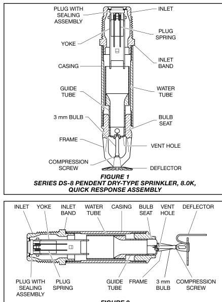
FIGURE 2 SERIES DS-8 HORIZONTAL SIDEWALL DRY-TYPE SPRINKLER, 8.0K, QUICK RESPONSE ASSEMBLY
