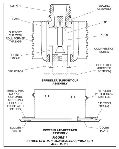
below. Down drafts through the sprinkler/support cup assembly can delay sprinkler operation in a fire situation.
