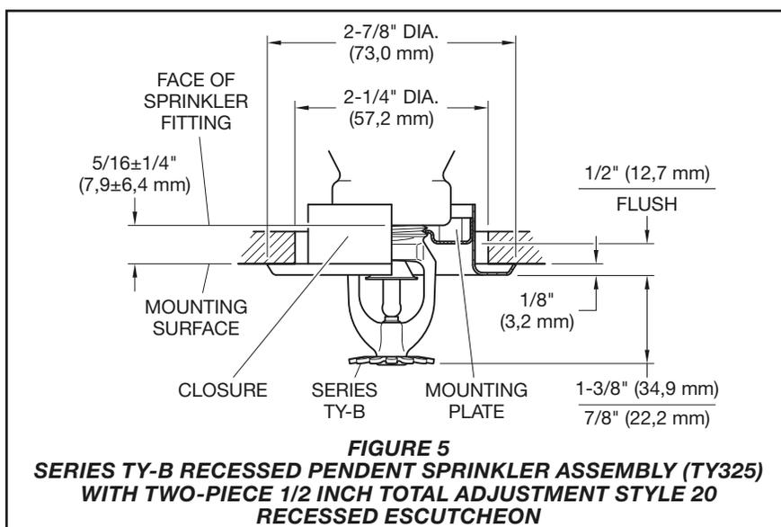
Automatic sprinklers are recommended to be inspected, tested, and maintained by a qualified Inspection Service in accordance with local requirements and/or national codes.
