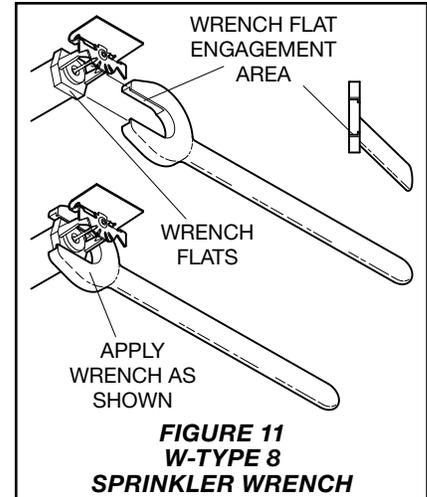
Close the fire protection system control valve and drain the system before removing the sprinkler.
