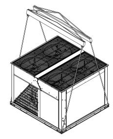
Figure 2: Typical Rigging
