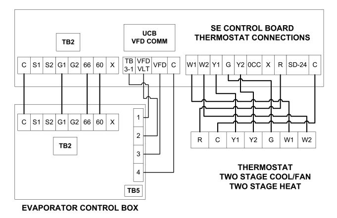
Figure 11: Typical Simplified Field Wiring Diagram – NM120 thru 240 Evaporator with YD120 thru 240 Condenser
