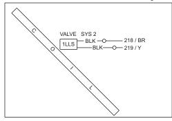
Figure 6: Typical NC300 Liquid Line Solenoid Wiring
