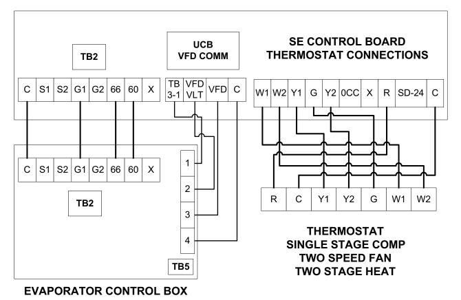
Figure 8: Typical Simplified Field Wiring Diagram – NL090 Evaporator with YC090/YE090 Condenser
