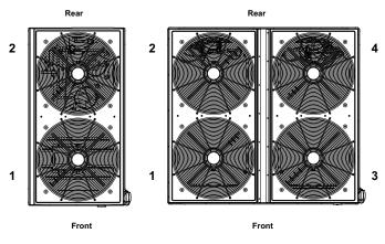
Figure 14: Fan Orientation - Control Box End
