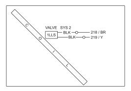
Figure 4: Typical NC120 - 240 Liquid Line Solenoid Wiring
