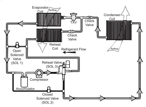
Figure 31: Cooling operation piping schematic - circuit #1 shown
