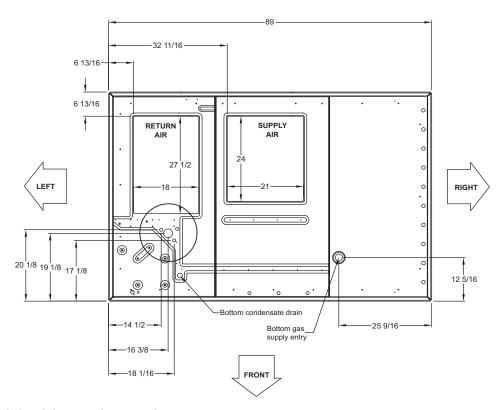
Figure 10: ZR078-150 unit bottom duct openings
