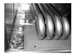
Figure 19: Discharge panel in place
