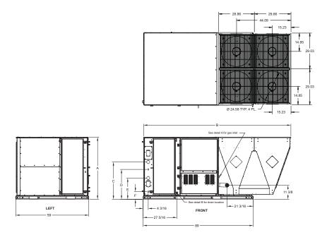
Figure 9: ZR150 physical dimensions
