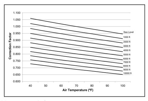
Figure 29: Altitude/temperature correction factors
