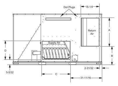
Figure 12: ZR078-120 unit side duct openings
