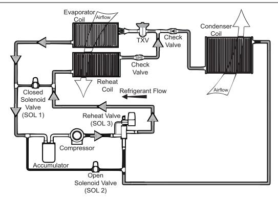
Figure 32: Reheat operation piping schematic - circuit #1 shown
