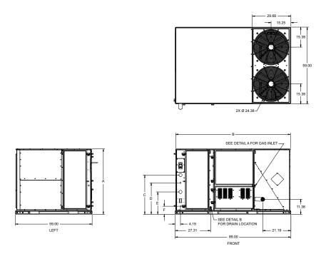
Figure 8: ZR078-120 physical dimensions
