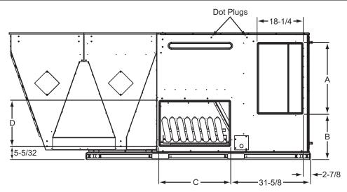
Figure 13: ZR150 unit side duct openings
