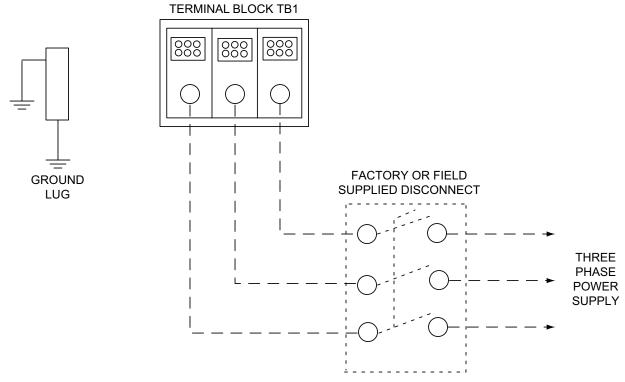
Figure 22: Typical field wiring disconnect - cooling unit with or without electric heat
