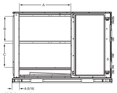
Figure 14: ZR078-150 unit/end left duct opening
