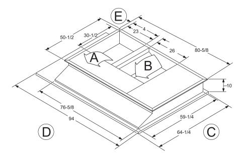
Figure 16: ZR078-150 transition roof curb
