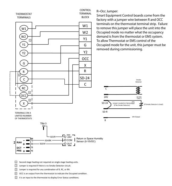
Figure 24: Typical low voltage field wiring
