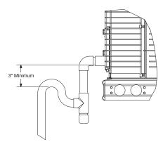
Figure 21: Condensate drain
