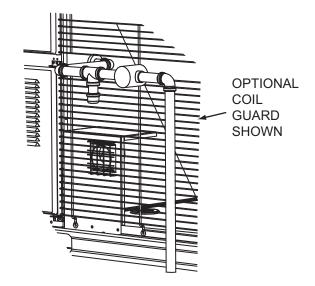
Figure 25: Side entry gas piping
