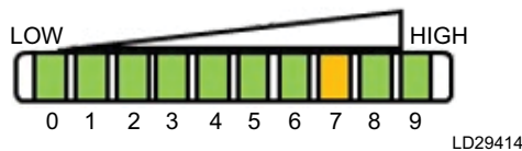
FIGURE 19 - FLOW SWITCH SET
