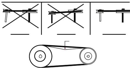
FIGURE 8: PULLEY ALIGNMENT & TENSION
