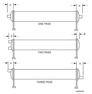
Table 32: Condenser nozzle dimensions, ft-in. (mm) vs design working pressure, psig (mpa)
