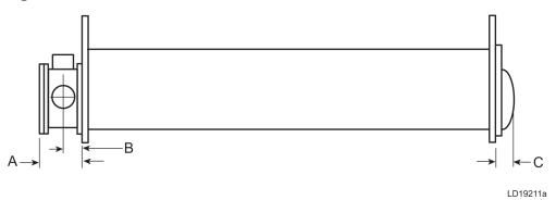
Table 29: Evaporator nozzle dimensions (1 and 2 pass), ft-in. (mm) vs design working pressure, psig (mpa)
