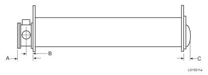
Table 34: Evaporator nozzle dimensions (1 and 2 pass), ft-in. (mm) vs design working pressure, psig (mpa)
