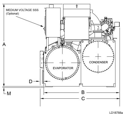
Figure 42: YK-EP Style B front view dimensions
