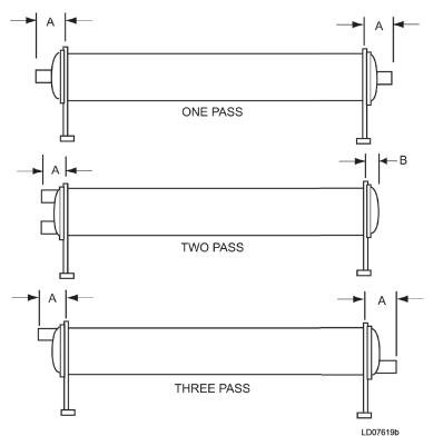
Table 27: Evaporator nozzle dimensions, ft-in. (mm) vs. design working pressure, psig (mpa)
