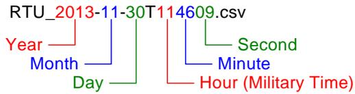
**Figure 10: Restoration File Name Structure**
