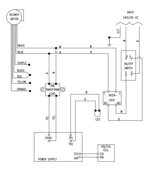
Figure 4 - Wiring Schematic 240V / 60Hz
