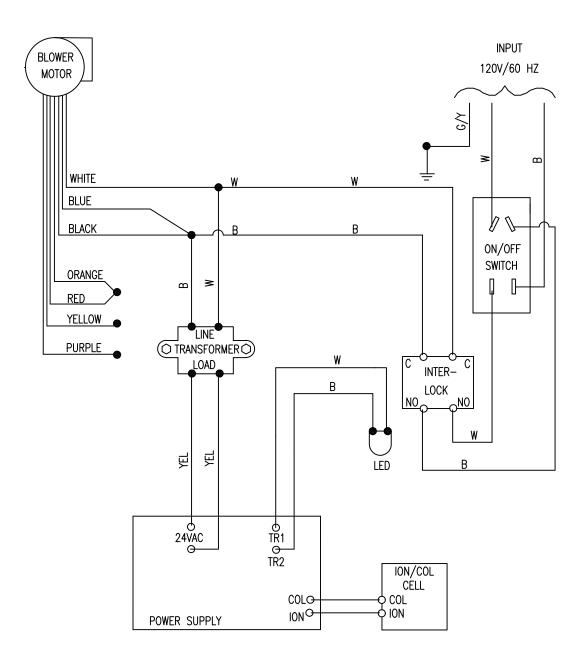
Figure 3 - Wiring Schematic 120V / 60Hz
