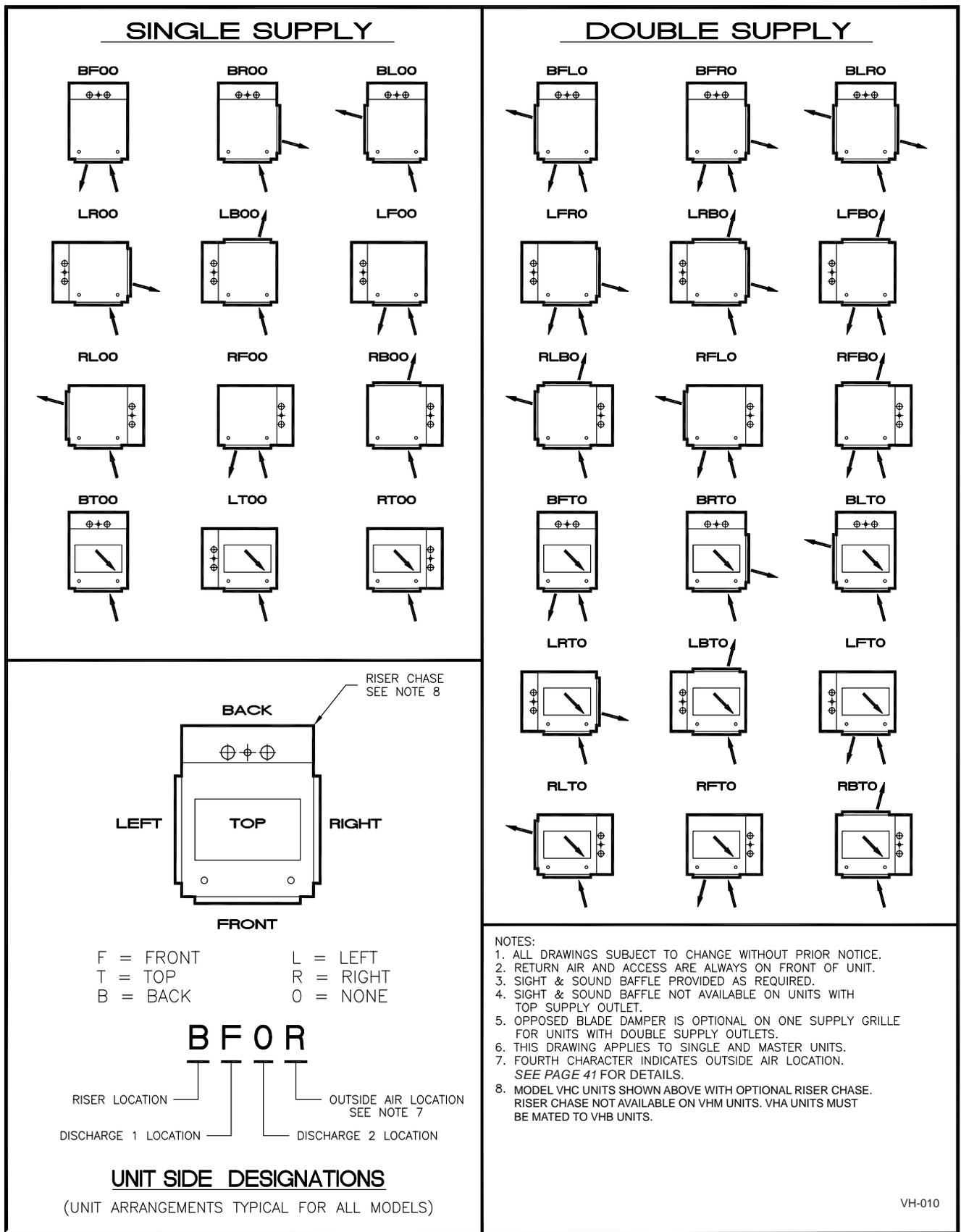
**FIGURE 23 - MODEL VHC/VHM/VHA VERTICAL HIGH RISE FAN COIL UNIT ARRANGEMENT DESIGNATIONS**
