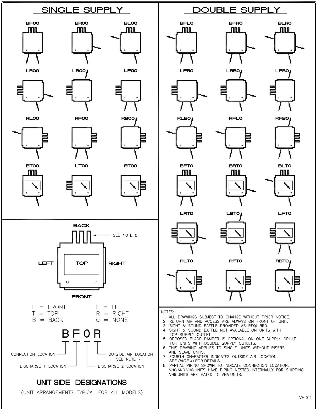
**FIGURE 24 - MODEL VHC W/O RISERS & VHS/VHB VERTICAL HIGH RISE FAN COIL UNITS, UNIT ARRANGEMENT DESIGNATIONS**
