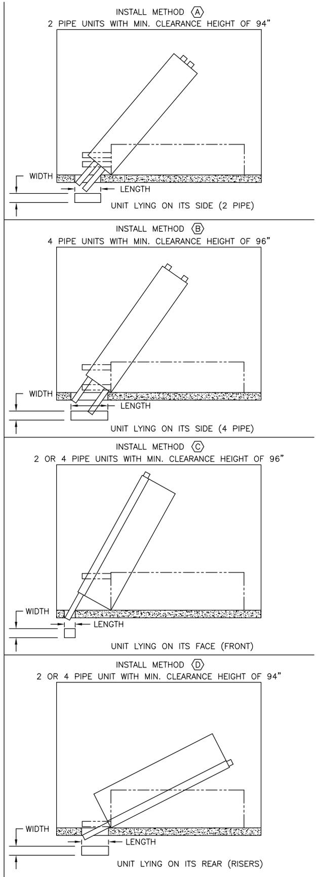
**FIGURE 32 - SUGGESTED RISER FLOOR OPENINGS VHC & VHM**
