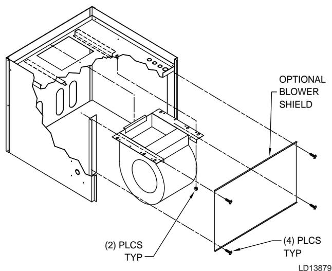
FIGURE 12 - MOTOR/BLOWER ASSEMBLY
