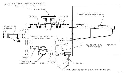
Optional Parts Supplied with Humidifier or Supplied by Others: Steam Valve Valve Actuator: Pneumatic, ON/OFF Electric, or Electric Modulating Actuators Inlet Strainer Supply Trap: F&T Trap or Inverted Bucket Trap
