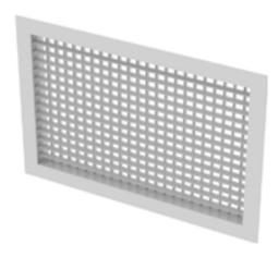
The AV and AVS supply grilles and registers are recommended for applications requiring noise reduction. They have individually adjustable, aerodynamically-shaped blades, and are available with front horizontal or front vertical blades. The grilles offer single and double deflection with 3/4" blade spacing.
