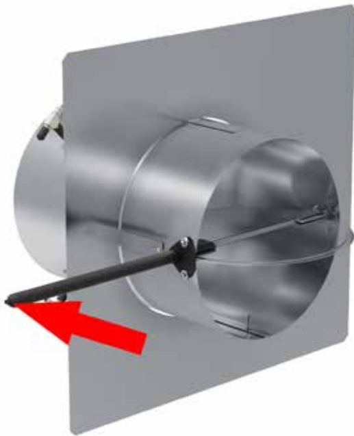
Damper shaft indicator in horizontal position, indicating fully open damper blade
