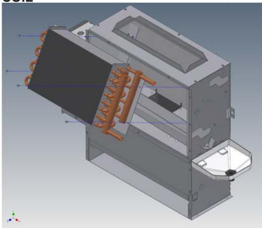
Remove screws to replace coil.
